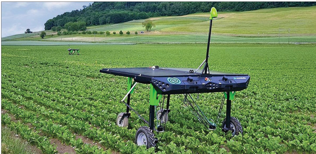
Slika 74. Autonomni robot za suzbijanje korova (Izvor: https://en.reset.org/these-smart-weed-killing-robots-use-twenty-times-less-herbicide-06272018/ ).
