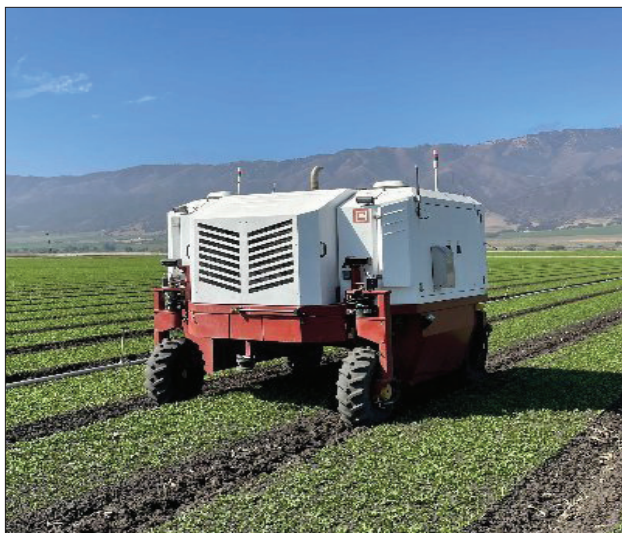
Slika 78. Laser robot (Izvor: https://vegetablegrowersnews.com/news/27m-secured-by-carbon-robotics-for-its-autonomous-field-weeders/ ) i Slika 79. Uništen korov (Izvor: https://blog.adafruit.com/2021/09/13/carbon-robotics-autonomous-weeder-zaps-weeds-with-lasers/ ).
