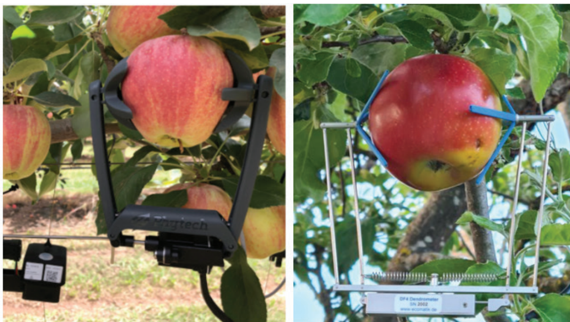
Slika 63. Izgled različitih tipova dendrometra za mjerenje promjera ploda (izvori: https://www.phytech.com/post/the-art-of-controlling-fruit-size i https://ecomatik.de/en/products/growth-and-plant-water-status-dendrometer/fruit-df/ )
