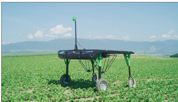
Slika 75. Solarni autonomni robot za suzbijanje korova (Izvor: https://ecorobotix.com/company/origins/ )
