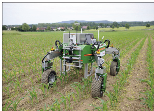
Slika 75. Solarni autonomni robot za suzbijanje korova (Izvor: https://ecorobotix.com/company/origins/ )
